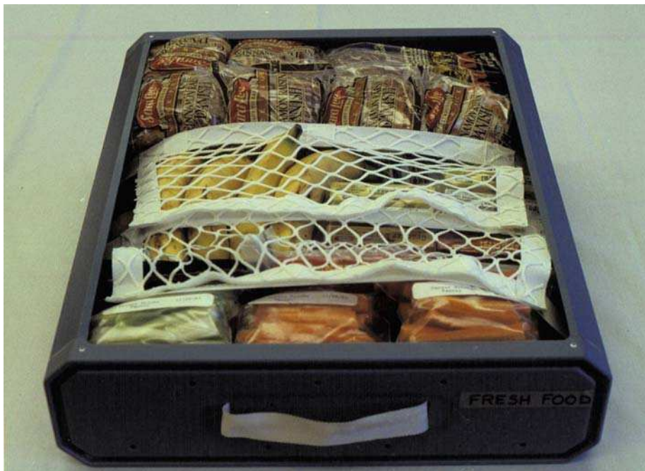
FIGURE 2.1 Shuttle fresh food locker tray with celery, carrots, bananas, and Danish rolls. Note the netting used to hold the food in place in microgravity (NASA photograph).
